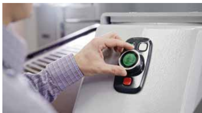
Control 5.0 in the SmartControl option consists of up to four SmartKnobs on the machine. These small displays allow users to access all relevant machine functions
