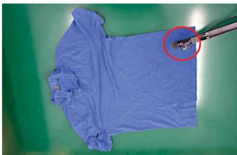
The AI uses a uEye XC camera to determine the type of material used in the textiles
