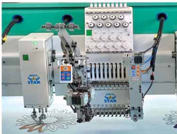
MIXED CHENILLE - HIGH SPEED CHAIN STITCH + HIGH SPEED FLAT EMB
